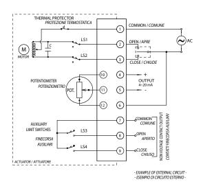
Allows to obtain a 4~20 mA output signal, proportional to the position of the actuator, in order to monitor the state of the valve.
