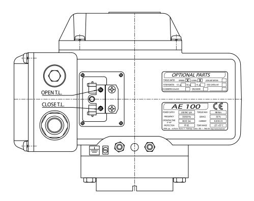
When ordering, please specify the torque value for which the limiters are to be set: the actuator is designed according to the customer's specifics before shipping, in order to ensure a perfect setting. However, if necessary, it is possible to adjust the set value by following the steps listed below.
