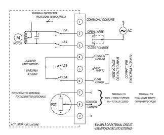
Allows to detect the actuator position in order to monitor the state of the valve.
